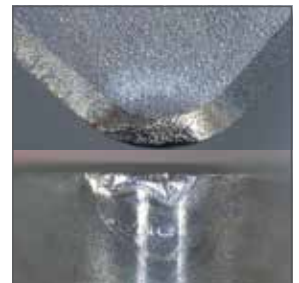
Competitor (uncoated) (After cutting 45 km)
