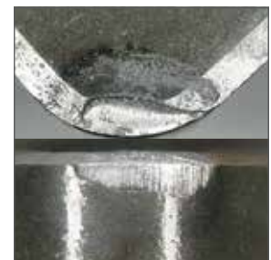
Conventional Tool (uncoated) (After cutting 0,5 km)
